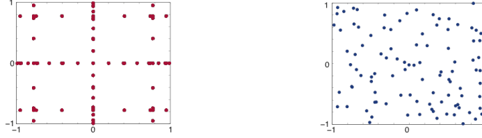
Figure 2: Smolyak sparse grid on the left and Monte Carlo sampling of the two-dimensional random vector on the right.
