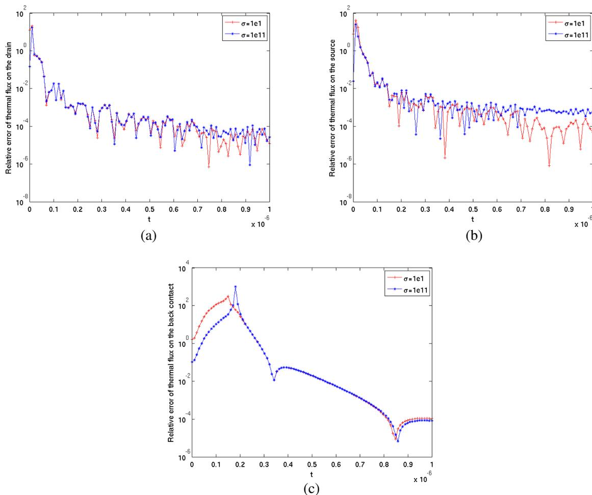
Figure 2: The evolution of the relative errors of the thermal outputs for extreme  $\sigma$ 's at  $t = 10^{-6}$  s. (a) Relative error of the thermal flux on the drain. (b) Relative error of the thermal flux on the source. (c) Relative error of the thermal flux on the back contact.
