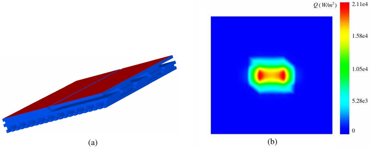
Figure 1: The Power-MOS device and its heat flux density on the back contact at  $t = 10^{-6}$  s. (a) Power-MOS device (the back contact is not shown). (b) Heat flux density on the back contact at  $t = 10^{-6}$  s.
